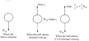
When the ball is just released, the net force on ball is  $W_{eff}$  (= mg - buoyant force)
