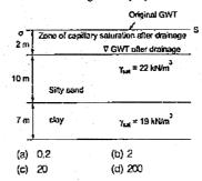
Q.24 In the situation shown in the given figure, the coefficient of permeability of the soil is 10<sup>-3</sup> cm/s. The discharge in one minute will be
