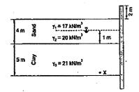
From the above diagram, the value of ellective stress at point X in kN/m2 is
