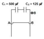
**639.** In the circuit shown in figure, find the charge on capacitor C<sub>2</sub> in steady state in μC.
