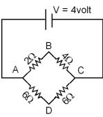
325. In fig the current through resistance (R) is
