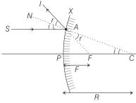
$\angle SAN = \angle PCA = i$  (corresponding angles)  $\angle NAI = \angle FAC = r$  (vertically opposite angles)
