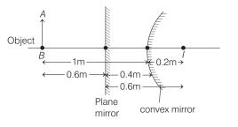
For plane mirror |u| = |v| = 0.6 m (3) For convex mirror, u = -1 m, v = +0.2 m (2) Use  $\frac{1}{f} = \frac{1}{v} + \frac{1}{u}$
