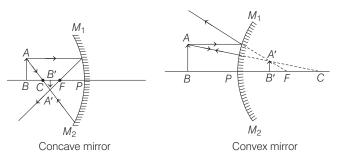
In concave mirror, A'B' is a real image while in case of convex mirror, A'B' is virtual.
