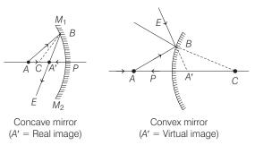
Another ray AB after reflection, will move along BE. In case of concave mirror, BE will intersect the principal axis at A. The two reflected rays BE and PA meet at A'. In image of A is formed at A'. In case of convex mirror, BE appears to intersect principal axis at A'. Reflected rays BE and PA appear to meet at A'. So image of A is formed at A'.
