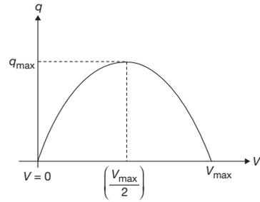
$V_{\max}$  = Free flow speed/free mean speed
