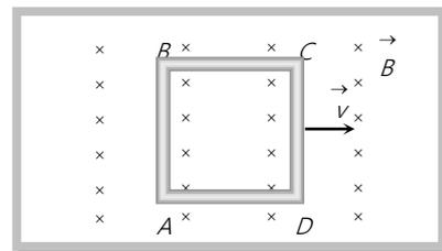
83. A conducting square loop of side  $l$  and resistance  $R$  moves in its plane with a uniform velocity  $v$  perpendicular to one of its sides. A magnetic induction  $B$  constant in time and space, pointing perpendicular and into the plane at the loop exists everywhere with half the loop outside the field, as shown in figure. The induced e.m.f. is
