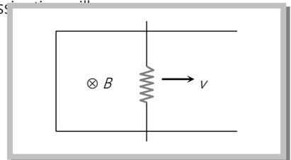
106. A rectangular loop on which a connector  $EF$  of length  $l$  slides, is lying in a perpendicular magnetic field. The induction of magnetic field is  $B$ . The resistance of the connector is  $R$ . If the connector moves with a velocity  $v$  then the current flowing in it will be
