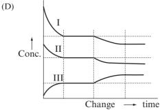
(S) Addition of inert gas at constant pressure
