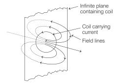
From the diagram of field lines, we can observe that whatever be the number of field lines emitted from coil, all of them goes back into the infinite plane only.
