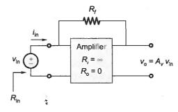
What is the value of input resistance,  $R_{in} = \frac{V_{in}}{i_{in}}$ ?
