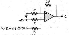
The output voltage  $V_{\alpha}$  for an input  $V_i = [2 + \sin(100t)] V$
