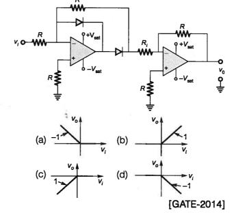
Q.29 In the figure assume the OP-AMPs to be ideal. The output  $v_0$  of the circuit is
