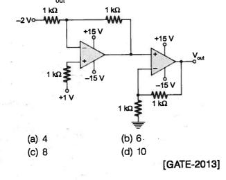
Q.15 Given that the op-amps in the figure are ideal, the output voltage  $V_0$  is
