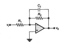
$R_2 = 159 \text{ k}\Omega$  $R_1 = 15.9 \text{ k}\Omega$  $C_1 = 1.0 \text{ nF}$
