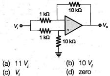
Q.11 Find  $V_0$  for the circuit shown below:
