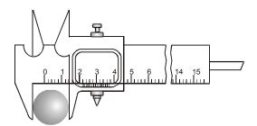
**Ex.** A vernier scale has 10 parts, which are equal to 9 parts of main scale having each path equal to 1 mm then least count =  $1 \text{ mm} - \frac{9}{10} \text{ mm} = 0.1 \text{ mm} [ \because 9 \text{ MSD} = 10 \text{ VSD}]$
