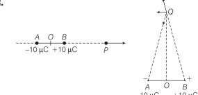
In given figures, OP = OQ = 15 cm, OA = OB = 2.5 mmMagnitudes of electric field at P and Q are respectively
