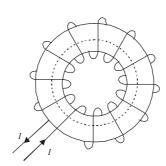
• The magnetic field produced in toroid will be same at all points on the circumference of the circle and at any point it will act along the tangent to the ring
