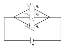
Total charge, q = q1 +q 2 +q3, q1 = C1.V, q2 = C2.V, q3 = C3.V
