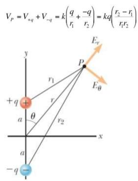
When r >> a, then  $r_1$ ,  $r_2$ and r are approximately equal and  $r_2$ -  $r_1 = 2acos\theta$ . Therefore,
