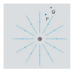
**Ans:** As V  $\alpha$  1/r , V<sub>P</sub> > V<sub>Q</sub>. Thus, (V<sub>P</sub> - V<sub>Q</sub>) is positive.
