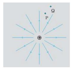
**Ans:** In moving a small positive charge from Q to P, work has to be done by an external agency against the electric field. Therefore, work done by the field is negative.
