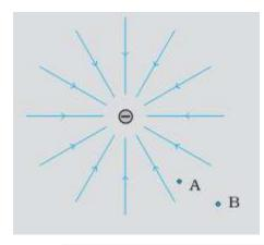
**Ans:** Due to force of repulsion on the negative charge, velocity decreases and hence the kinetic energy decreases in going from B to A.(Potential energy increases)
