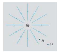
**Ans:** Potential energy difference of a small negative charge between the points A and B =  $U_A - U_B = -q (V_A - V_B)$
