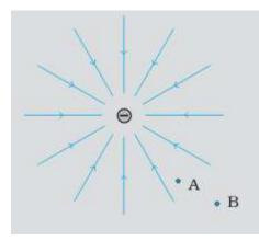
**Ans:** Work done = potential energy difference of a small negative charge between the points A and B =  $U_A - U_B = -q (V_A - V_B)$
