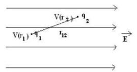
PE of the system of charges is the total work done to assemble the charges from infinity.
