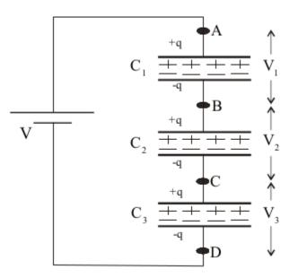
If V 1,V 2 and V 3 are the pd's of capacitors respectively,
