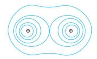
Que 15: Draw the equipotential surface for an electric dipole? *Marks :(1)* Ans:
