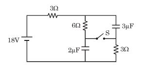
(A) Charge on  $2\mu$ F before the switch is open is  $9\mu$ C
