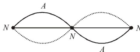
A node is a place of zero amplitude and an antinode is a place of maximum amplitude.
