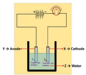
Note: Electrodes are the good conductors of electricity from which electric current enters or leaves the circuit. The electrode connected with the positive terminal of the battery is called the anode and the electrode connected with the negative terminal of the battery is called the cathode.
