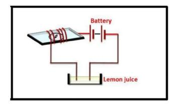
When a weak or strong electric current conducts through the liquid in the circuit shown the magnetic needle of the compass show deflection.
