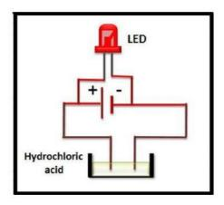
The longer lead of the LED is connected to the positive terminal of the battery and the shorter lead is connected to the negative terminal.
