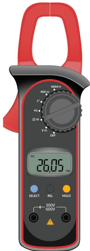
A tong tester is shown in figure 6.13. Ammeters cannot be used directly to
