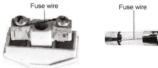
It is an alloy of lead and tin (37% lead + 63% tin). It has a low resistivity and low melting point. As soon as the safe limit of current exceeds, the fuse "blows" and the electric circuit is cut off.
