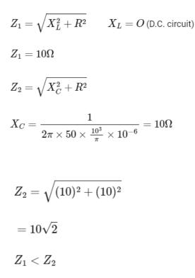
**Question:** The maximum power is dissipated for an ac in a/an:
