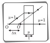
$\Delta x = Apparent normal shift = t \left(1 - \frac{1}{\mu}\right)$
