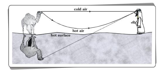
Similar to 'mirage' in deserts, in polar regions 'looming' takes place due to TIR. Here  $\mu$  decreases with height and so the image of an object is formed in air if (i> $\theta_c$ ) as shown in figure.
