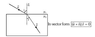
(ii) The product of refractive index and sine of angle of incidence at a point in a medium is constant.  $\mu_1 \sin i = \mu_2 \sin r$  (Snell's law)
