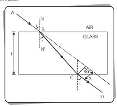
Lateral shift  $x = \frac{t \sin(i - r)}{\cos r}$ ; t = thickness of slab
