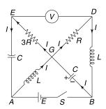
After opening the switch, the current in R and the inductor between B and D must be same (since voltmeter does not conduct). It implies that current through R is still I and  $V_G - V_D = RI = E$
