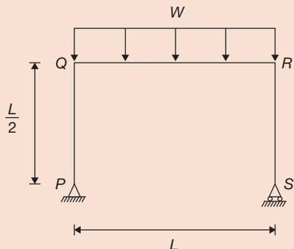
The bending moment in the beam at the joint 'Q' is
