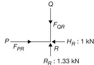
$$F_{PR} = 1 \text{ kN(C)} \quad F_{QR} = 1.33 \text{ kN(C)}$$
