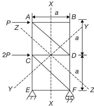
Out of the three sections  $X-X$ ,  $Y-Y$ ,  $Z-Z$ , section  $Z-Z$  is effective since the number of unknown forces are only three. Considering the equilibrium of above cut part.
