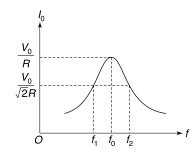
**21.** Current amplitude at resonance frequency  $(\omega_0)$  is  $I_0 = \frac{V_0}{R}$
