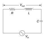
**Q. 20:** In a series LCR circuit, the frequencies at which the current amplitude is  $\frac{1}{\sqrt{2}}$  times the current amplitude at resonance are  $f_1$  and  $f_2(>f_1)$ . Find the frequency bandwidth of resonance which is defined as  $\Delta f = f_2 - f_1$ . Express your answer in terms of R and L. Assume that resonance
