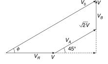
With  $\omega_0 = 4 \times 10^5$  rad s<sup>-1</sup>, the circuit is in resonance (:  $V_L = V_C$ )
