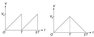
**Q. 4:** A voltage waveform is as shown in the Figure calculate the ratio of rms value and average value of the voltage.
