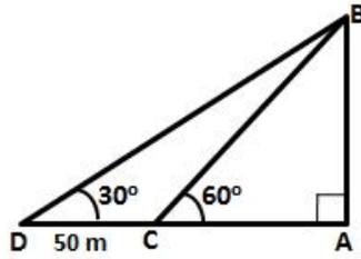
Let AB be the tree and AC be the width of the river. Let D be a point such that CD = 50 m. Given that  $\angle BCA = 60^\circ$  and  $\angle BDA = 30^\circ$ .
