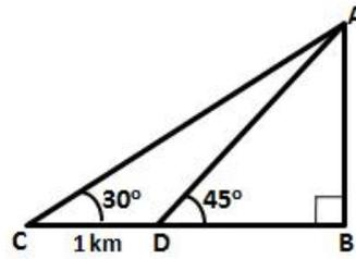
Let AB be the hill of height 'h' km and C and D be the two consecutive stones such that  $CD = 1$  km,  $\angle ACB = 30^\circ$  and  $\angle ADB = 45^\circ$ .
