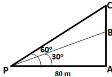
Let AB be the unfinished tower and C be the top of the tower when finished. Let P be a point 80 m from the foot A. In  $\triangle BAP$ ,
