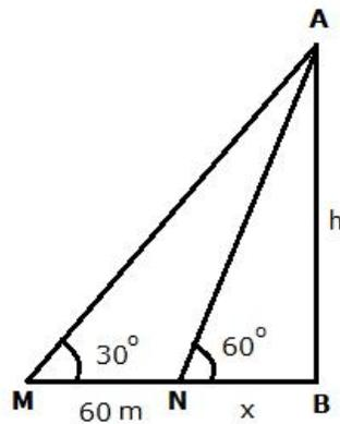
Let AB be a building and M and N are the two positions of the man which makes angles of elevation of top of building as  $30^\circ$  and  $60^\circ$  respectively.
