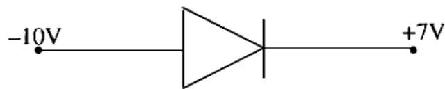
Is the Junction diode D is forward or reverse biased, in the given diagram
