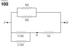
In the circuit shown, the current through the  $4\Omega$  resistor is 1Awhen the points P and M are connected to a DC voltage source. The potential difference between the points M and N is
