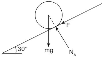
The initial kinetic Energy ( $K.E_1$ ) decreases to final  $K.E_2 = 0$  at the top of the travel. The only force that does work in the component (negative) of the weight  $W$  along the plane.
