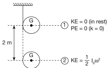
$$\begin{aligned} \frac{1}{2} I_0 \omega^2 &= mg(2) \\ \Rightarrow \frac{1}{2} \left[ \frac{mr^2}{2} + mr^2 \right] \omega^2 &= 30 \times 9.81 \times 2 \\ \Rightarrow \frac{1}{2} [1.5 \times 30 \times 0.5^2] \times \omega^2 &= 30 \times 9.81 \times 2 \\ \Rightarrow \omega &= 10.23 \text{ rad/s} \\ V_G &= \omega \times r = 10.23 \times 0.5 = 5.115 \text{ m/s} \quad \text{Choice (A)} \end{aligned}$$
