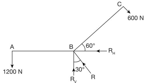
$$\begin{aligned} R_H &= F \cos 30^\circ = 600 \times \cos 30^\circ \\ &= 519.615 \text{ N} \\ \text{and } R_V &= F \sin 30^\circ + 1200 \\ &= 600 \times \sin 30^\circ + 1200 \\ &= 1500 \text{ N} \end{aligned}$$
