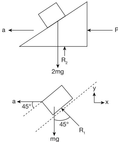
$$\begin{aligned} \Sigma F_x = ma_x &\Rightarrow -P = 2m(-a) \\ \Rightarrow P &= 2ma \\ \Sigma F_x = ma_x & \\ \Rightarrow m(-a) &= -R_1 \sin 45^\circ \quad \rightarrow (1) \\ \Sigma F_y = ma_y &\Rightarrow R_1 \cos 45^\circ = mg \\ \Rightarrow R_1 &= mg / \cos 45^\circ \quad \rightarrow (2) \end{aligned}$$
