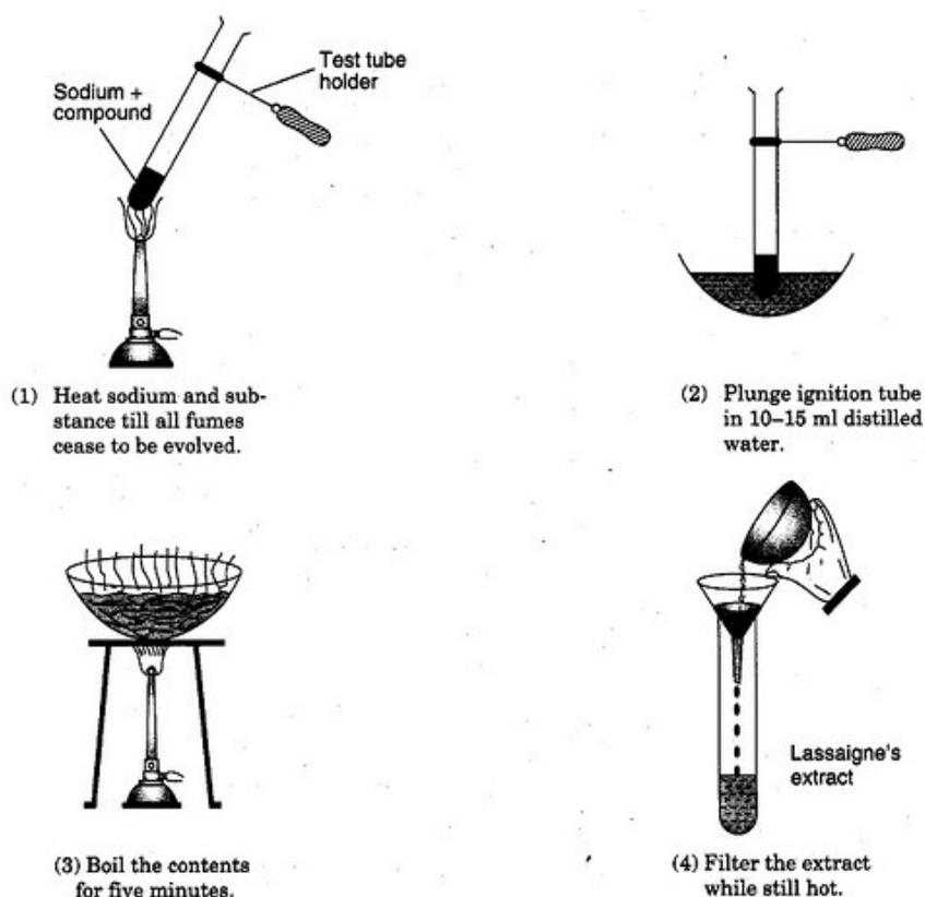
Fig. 10.1. Preparation of Lassaig's extract.
