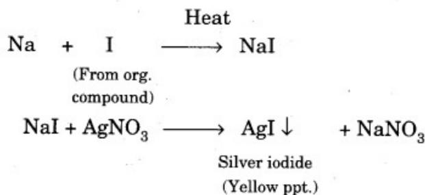
The function of adding conc.  $\text{HNO}_3$  and boiling is to decompose any sodium cyanide or sodium sulphide present in the extract. Otherwise these compounds will interfere with the tests of halides since  $\text{NaCN}$  gives a white ppt. with silver nitrate while  $\text{Na}_2\text{S}$  gives a black ppt.
