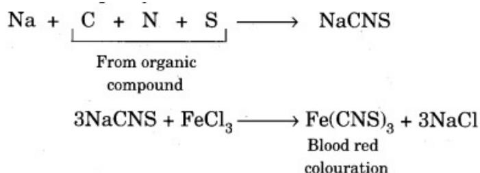
Thus, appearance of a blood red colouration on performing Lassaigne's test for nitrogen indicates the presence of both nitrogen and sulphur in the organic compound.
