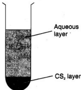
**Fig. 10.2.** Carbon disulphide test.
