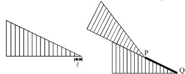
In this diagram, we are interested in measuring the length of the line PQ. If both the inclines are identical and their angles are equal to  $\theta$  then what is the least count of the instrument.
