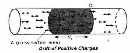
2. Let 'V<sub>d</sub>' be the drift speed of the charges and 'n' be the number of charges present in the conductor in an unit volume.
