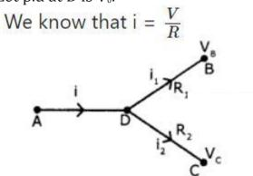
$$i = \frac{V}{R} = \frac{V_A - V_0}{R} = \frac{70 - V_0}{10}$$
