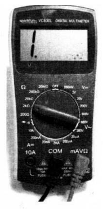
Display: The display usually has four digits and the ability to display a negative sign.
