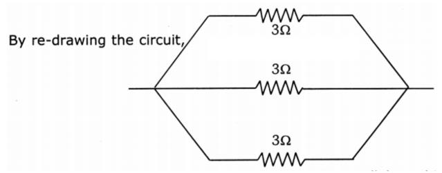
From the above circuit, all the resistors are in parallel combination
