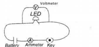
2. Close the circuit and note the readings of ammeter (I) and voltmeter (V) tri the following table.
