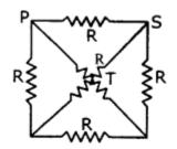
The circuit diagrams for the given arrangement is along PTR and QTS Is ineffective as no current flow through it.
