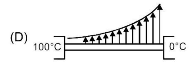
12. A metal rod of cross-sectional area 1.0 cm<sup>2</sup> is being heated at one end. At one time, the temperature gradient is 5.0°C/cm at cross-section A and is 2.6 °C/cm at cross-section B. Calculate the rate at which the temperature is increasing in the part AB of the rod. The heat capacity of the part AB = 0.40 J/°C, thermal conductivity of the material of the rod = 200 W/m-°C. Neglect any loss of heat to the atmosphere.
