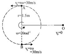
$$r = 1.5 \text{ m (given)}; \ \omega = 20 \text{ rads}^{-1} \text{ (given)}$$
