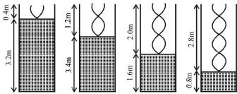
or heights of water level are (3.6 - 0.4) m, (3.6 - 1.2) m, (3.6 - 2.0) m and (3.6 - 2.8) m.
