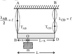
For rotational equilibrium of massless rod, taking torque about point O.
