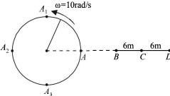
$\Rightarrow$  When the detector is at C moving towards D, the source is at  $A_1$  moving leftwards. It is in this situation that the frequency heard is minimum
