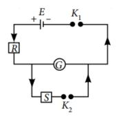
Resistance of galvanometer by half deflection method.
