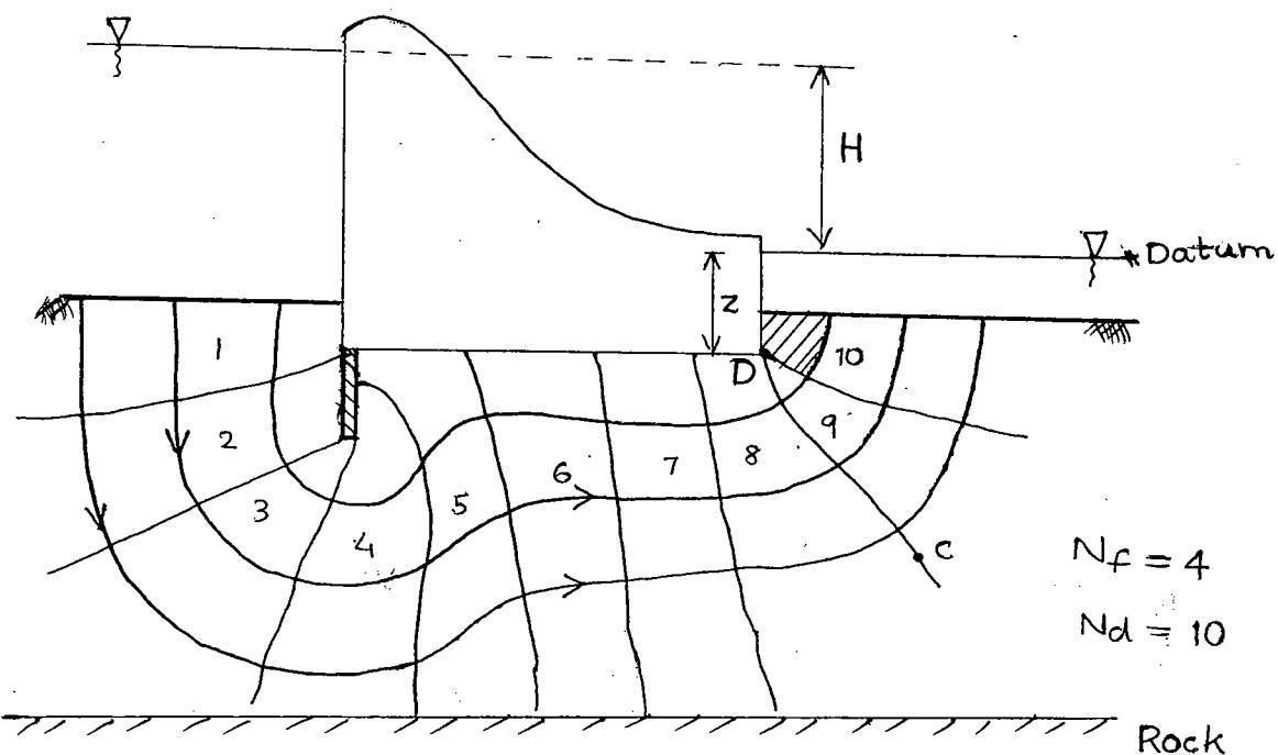
$H$  = seepage head (or) head causing flow. (or) total head loss
