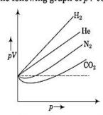
Find out for which gases compressibility factor  $(\mathbf{Z})$  is greater than 1
