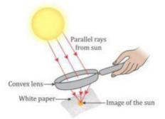
Focus the light coming from the Sun on the paper by adjusting the distance between the convex lens and the paper till a bright and sharp spot of light is obtained on the paper. This bright spot obtained on the paper is the image of the Sun formed by the convex lens.
