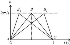
So, the | acceleration | must be greater than or equal to  $4 \text{ m/s}^2$  at some point or points in the path.
