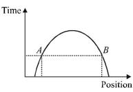
As shown, at a given instant of time, the body is at two different positions A and B which is not possible.
