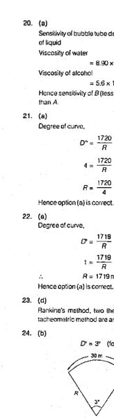
Sensitivity of bubble tube depends upon viscosity of liquid
