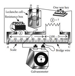
According to wheatstone bridge principle, at the null point.
