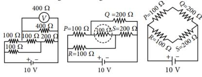
$\Rightarrow$  Voltmeter measures voltage across Q as  $\frac{200}{300}(10 \text{ V}) = \frac{20}{3}$
