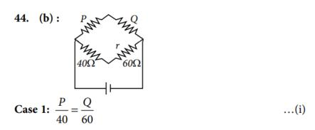
On shunting Q with 50  $\Omega$ , the resistance of the arm containing Q comes down, so length also must shorten to keep the ratio same.
