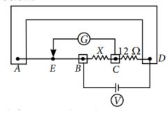
**46. (b)**: No deflection in the galvanometer means wheatstone bridge is balanced. So,  $\frac{X}{12} = \frac{R_{BJ}}{R_{AJ}}$
