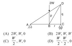
**15.** For the truss shown in the figure, the force in member AB is
