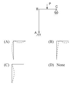
**26.** Rotational stiffness coefficient,  $K_{11}$  at joint 'C' for the frame having two members of equal  $\frac{EI}{\ell}$  is given by
