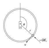
(b) The circular motion needs a radial force equal to  $mv^2/r$ .
