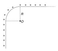
**Q. 53:** (a) There is a long uniformly charged cylinder having a volume charge density of  $\rho$  C/m<sup>3</sup>. Radius of the cylinder is R. Find the electric field at a point at a distance x from the axis of the cylinder for following cases
