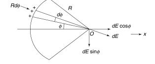
Due to symmetry field is along x only. We need to add all  $dE \cos \phi$  components.
