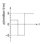
**Q. 58:** There are two infinite slabs of charge, both of thickness d with the junction lying on the plane x = 0. The slab lying in the range 0 < x < d has a uniform charge density  $+\rho$  and the slab lying in the region -d < x < 0 has uniform
