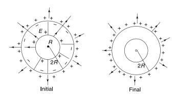
In initial configuration there is electric field in all region r > R. The field varies as  $E = \frac{1}{4\pi \epsilon_0} \frac{Q}{r^2}$ . In final configuration there is no field in the region R < r < 2R. Elsewhere the field is similar to that in initial configuration. Thus initial configuration has more energy stored in electric field given by
