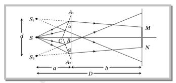
Let the separation between  $S_1$  and  $S_2$  be d and the distance of slits and the screen from the biprism be a and b respectively *i.e.* D = (a + b). If angle of prism is  $\alpha$  and refractive index is  $\mu$  then  $d = 2a(\mu - 1)\alpha$
