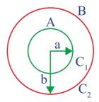
It consists of two concentric spherical shells as shown in figure. Here capacitance of region between the two shells is  $C_1$  and that outside the shell is  $C_2$ . We have  $C_1 = \frac{4\pi \in_0 ab}{b-a}$  and  $C_2 = 4\pi \in_0 b$ .
