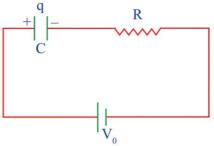
Discharging of a capacitor:  $q = q_0 e^{-t/RC}$
