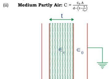
When a di-electric slab of thickness t & relative permittivity  $\epsilon_r$  is introduced between the plates of an air capacitor, then the distance between the plates is effectively reduced by  $\left(t - \frac{t}{\epsilon_r}\right)$  irrespective of the position of the dielectric slab.
