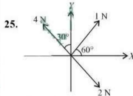
Three forces acting on a body are shown in the figure. To have the resultant force only along the  $y$ -direction, the magnitude of the minimum additional force needed is
