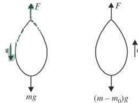
Let mass  $m_0$  be removed from the balloon so that it starts moving up with an acceleration  $a$ . Then,
