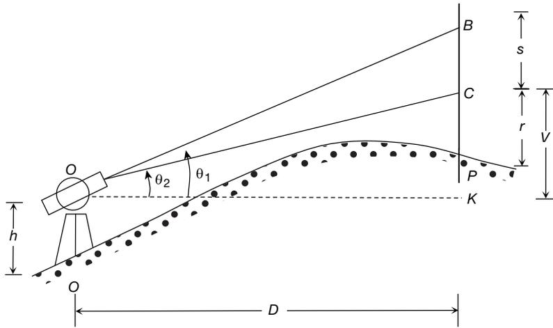
**Tangential method (elevation angles)**
