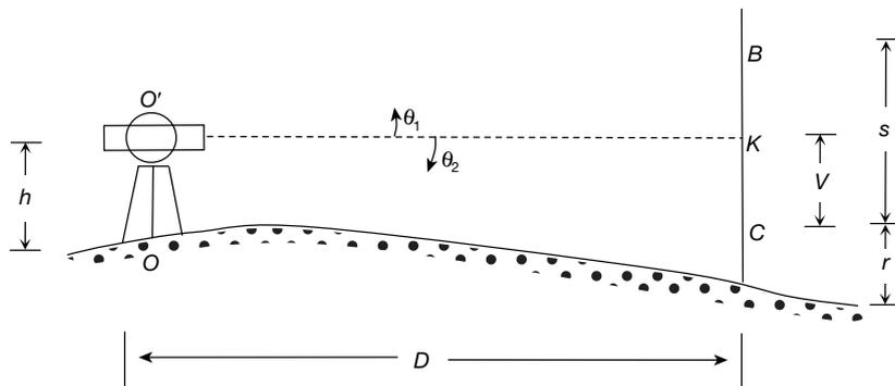
**Tangential method (one angle of elevation and the other angle of depression)**
