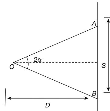
**Tangential Method** In this method, tacheometry observations are made for vertical angles and staff intercepts are obtained by the cross-wires only. Stadia wires are not used at all. This method of tacheometry is similar to the method of trigonometrically levelling. It is used when theodolite is not fitted with stadia wires.
