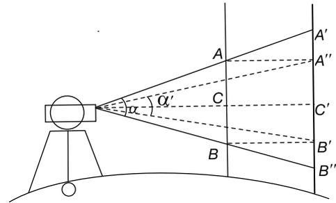
When the parallax angle  $\alpha$ , defined by means of stadia wires, is kept fixed and staff intercept is varied, this method is called fixed hair method. In this method, the distance and elevation for horizontal sights is given by
