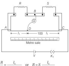
$$\frac{R}{S} = \frac{l_1}{(100 - l_1)} \quad \text{or} \quad R = S \ \frac{l_1}{100 - l_1}$$
