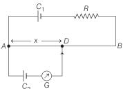
Statement II At the balance point, the potential difference between AD due to cell  $C_1 = E_2$ , the emf of cell  $C_2$ .
