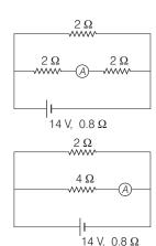
$$\begin{array}{l} Total\ resistance\ of\ the\ circuit \\ = \frac{2\times 4}{2+4}+\ 0.8 = \frac{8}{6}+\ 0.8 = \frac{12.8}{6}\ \Omega \end{array}$$
