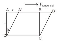
ABCD is the shape of body, before we apply tangential force and A'B'CD is the shape of body after applying tangential force.
