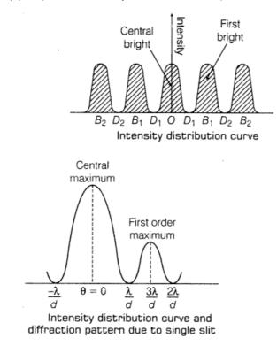
The intensity of bright fringes in interference is same for all the bright fringes whereas in diffraction pattern, the central fringe is brightest and intensity of secondary maxima decreases with the increase of their order.
