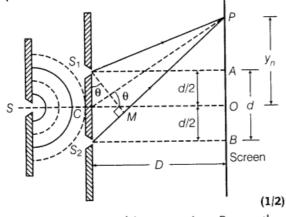
Considering any arbitrary point *P* on the screen at a distance  $y_n$  from the centre *O*. The path difference between interfering waves is given by  $S_2P - S_1P$
