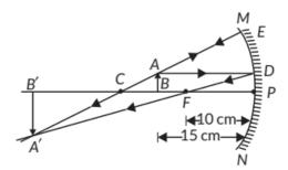
From ray diagram, v = -30 cm, i.e., beyond C Nature of image is real, inverted and magnified.
