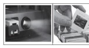
There is a tray where the slides are to be put into a particular orientation so that the viewers can see the enlarged erect images of the transparent slides. This means that the slides will have to be inserted upside down in the projector tray. To show her students the images of insects that she investigated in the lab, Mrs. lyer brought a slide projector. Her slide projector produced a 500 times enlarged and inverted image of a slide on a screen 10 m away.
